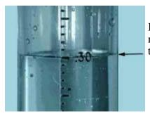
In this picture, we see an illustration of the calibrated measurement tube in the rain gauge that contains three tenths (thirty hundredths) of an inch. 0.30 inches
