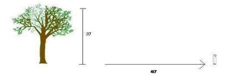
The gauge should be twice as far away from an object as that object is tall. In this picture, the tree is 20 feet tall, so the gauge is 40 feet away.
