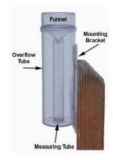
distance away from obstacles like buildings or trees. As a rule of thumb, if a tree is 40 ft. tall, the gauge should be placed at least 80 ft. downwind from it. This will help avoid potential blockage of the gauge. It is not always possible to find the perfect location. If in doubt, do your best!
