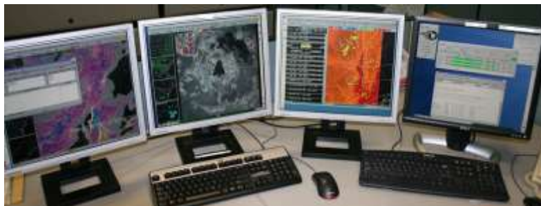
AWIPS display monitors, 3 for graphics, one for text.
