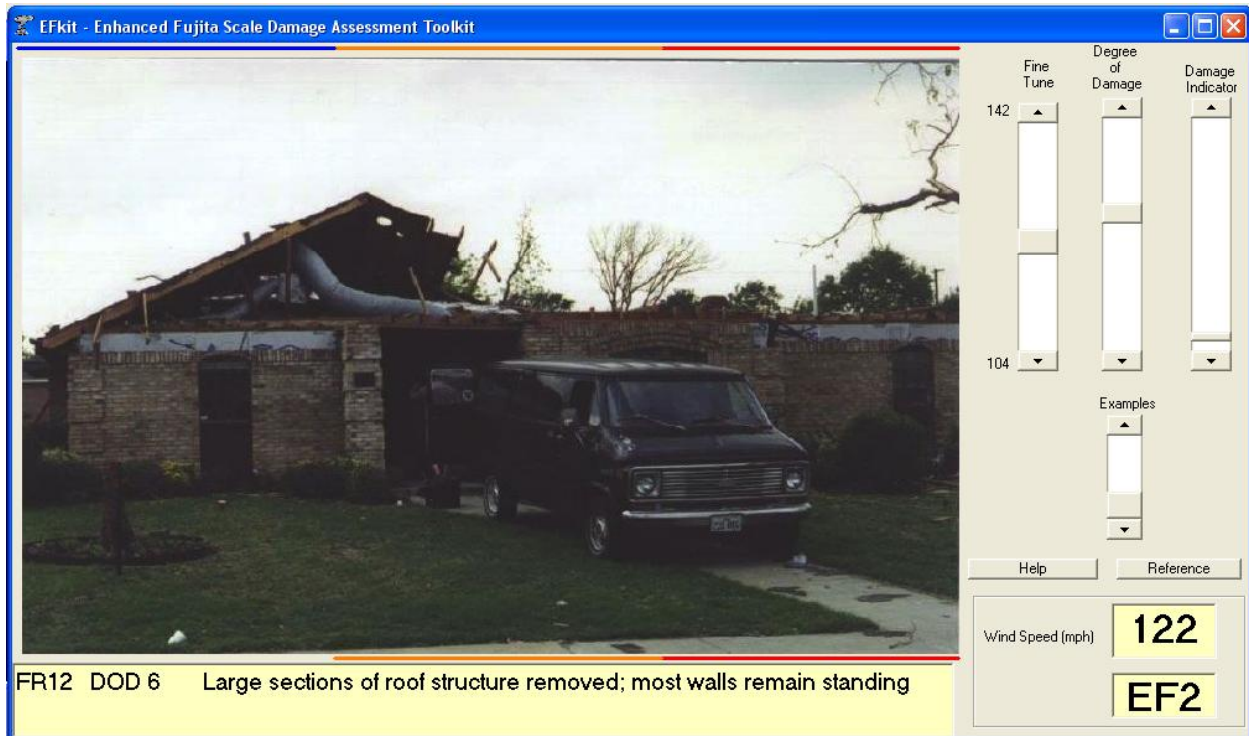
Fig. 4. An example of EFkit guidance. The Damage Indicator (DI) and Degree of Damage (DoD) can be set by slide bars, and the results fine-tuned based on the particular damage observed. Photographs accompany many of the DIs and DoDs for comparison.
