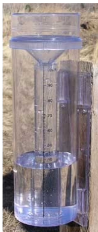
The rain gauge used by CoCoRaHS observers is a plastic tube that is easily mounted.
