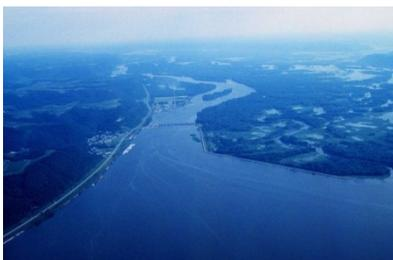
The US Army Corps of Engineers maintains a Lock and Dam (#8) at Genoa, WI that is used to manage navigational water levels, not for flood control.
