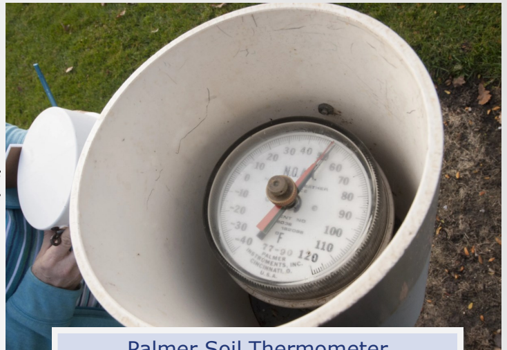
Palmer Soil Thermometer
