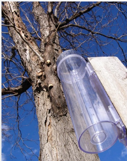
Rain gauge under a tree (bad)
