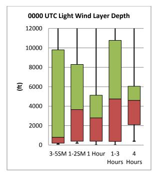
**Fig. 14.** Box-and-whiskers plot of the light wind layer depth (10 knots or less) for each fog category at 0000 UTC. Each "box" represents the inter-quartile range (25<sup>th</sup> to 75<sup>th</sup> percentile) with the horizontal line through each box signifying the median value. The top and bottom of the "whiskers" represent the maximum and minimum depth for each category. For some fog categories, the maximum depth exceeds the top value on the plot.
