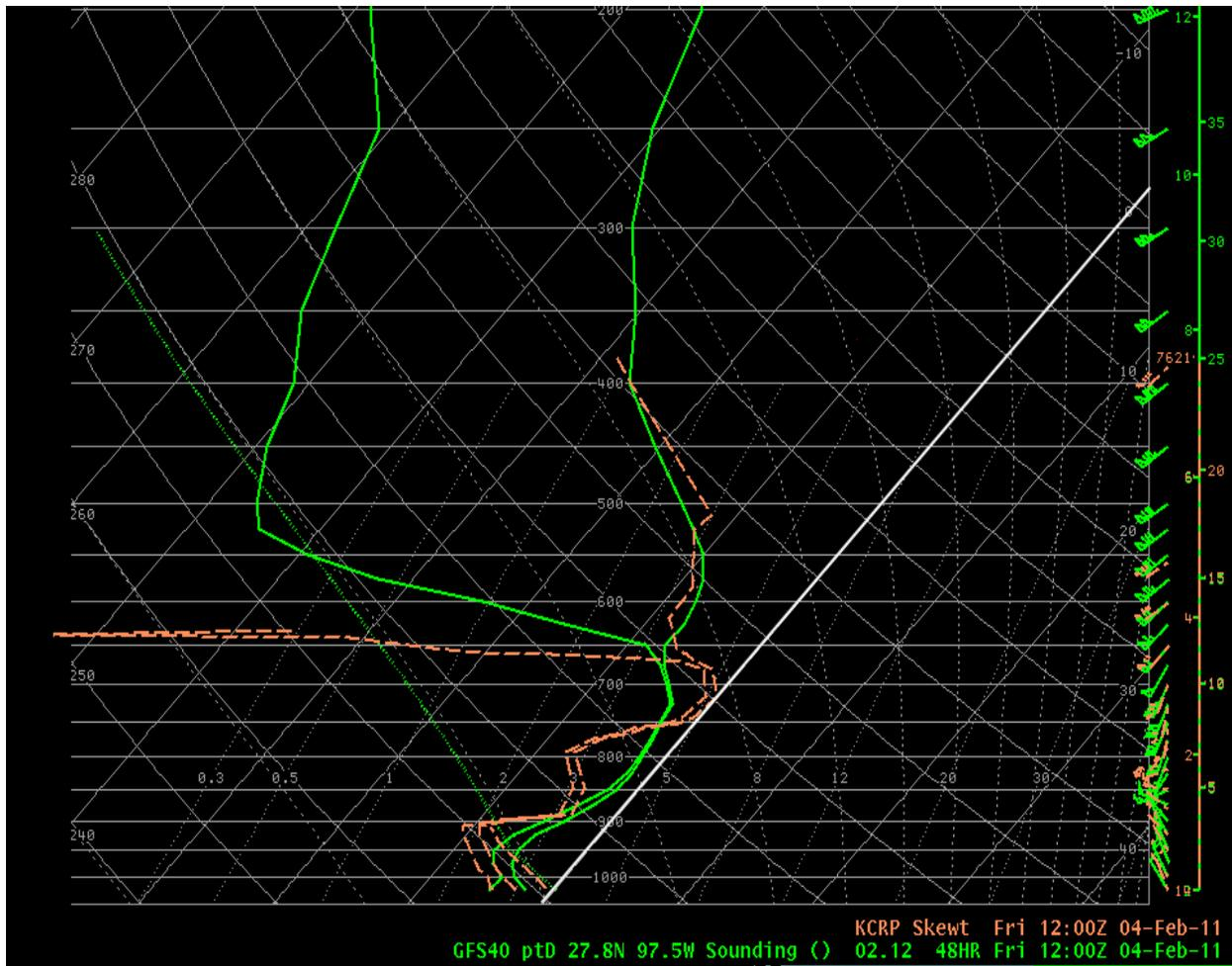
**Fig. 9-2: Same as Fig. 9-1, except at 1200 UTC 4 Feb. There is a loss of observed sounding data above 400 mb as the radiosonde failed due to significant icing.**
