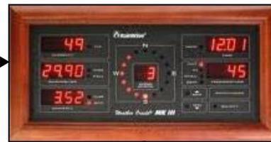
The Console/Display can be connected to a Personal Computer for data archiving using manufacturer-provided or third-party software.
