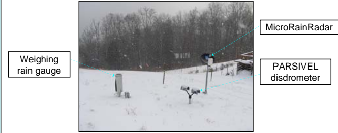
Figure 2: Precipitation instruments during a light snow event
