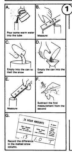
At the beginning of the snowfall season only the 8-inch gage can is exposed to catch the snow. The funnel and measuring tube are removed at the beginning of the snowfall season. The measuring tube is used to measure the water from the melted snow.
