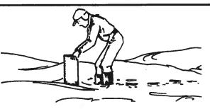
4. If the snow has blown out of the can or the "catch" is not good, cut a "biscuit" with the can where the snow is near the average and melt the biscuit for the water equivalent.
