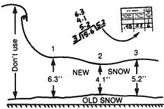
3. When possible, take several measurements where the snow is least affected by drifting (don't include deep drifts) and average.
