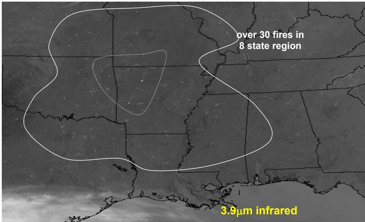
**Figure 3.** MODIS natural color composite image (top) and 3.9μm infrared image (bottom) for March 24, 2003. The color image highlights smoke plumes while the infrared image identify "hot spots" at the surface.
