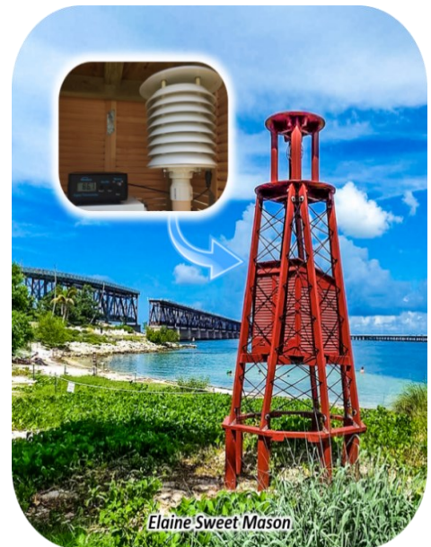
The new Bahia Honda temperature sensor is harbored in a lighthouse structure that is solar-powered.
