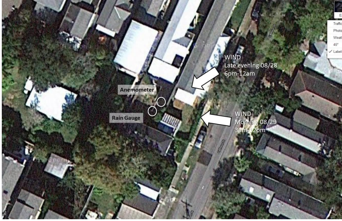
1521 Figure 34. Aerial imagery showing location of Weather Underground PWS site KLANEWOR15 1522 in relation to nearby trees and buildings. The predominant wind direction during the heaviest 1523 period of rainfall, roughly 3 AM-2PM on August 29 th , 2012, was from the east, which likely 1524 caused an under-estimate. 1525
