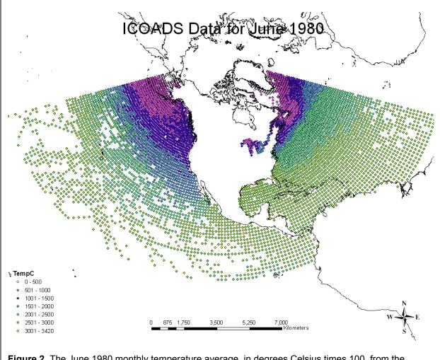
**Figure 2.** The June 1980 monthly temperature average, in degrees Celsius times 100, from the ICOADS data. Data points are every 1-degree falling on lines of whole degrees latitude and longitude. This example shows that data were not always available in every grid box.
