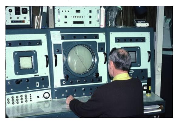
This is a 1980s era photo of the WSR-57 console at the National Weather Service at MSP. By this time, it had a system by which radar echoes were digitally processed. In 1965, however, there was no such digital processing, and one had to apply manual attenuation so that the operator could see some of the finer detail of critical echoes. The radar operator on May 6 was very skilled at this, enabling one to see great detail, including a number of hook echoes.
