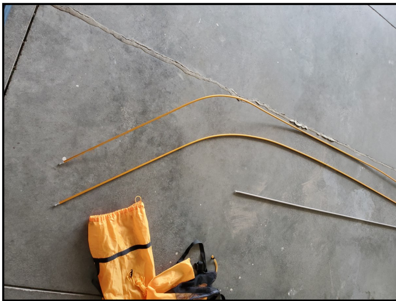
These tent poles were broken when a tent was blown away by a strong thunderstorm. Photo Credit: Darren Snively
