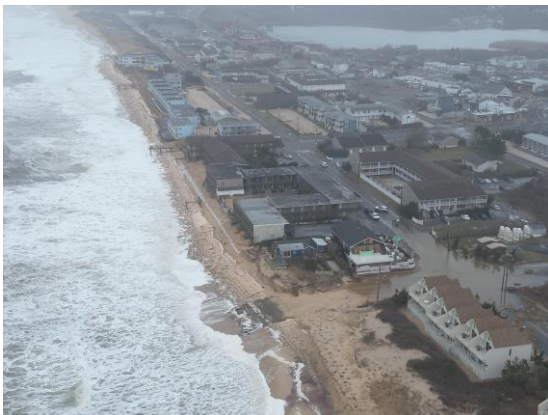
Montauk – One oceanfront home destroyed. Overwash and inundation onto several streets across the south shore of Montauk, including South Emerson Ave.
