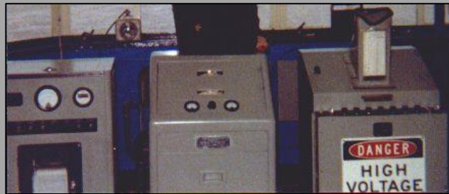
Transmissometer Readout (visibility machine), temperature/dew point readout, Rotating Beam Ceilometer (ceiling height) readout
