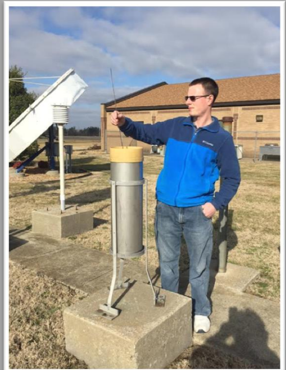
Here is a photograph of one of our Meteorologist Interns (Sean Poulos) measuring precipitation from a standard 8 inch rain gage behind the NWS Paducah office.
