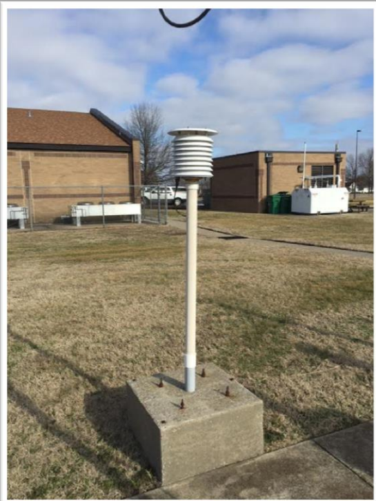
A Max/Min Temperature System (MMTS) used to measure temperature. It connects to a display box inside a residence or business so the observer can read the data from inside.
