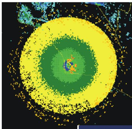
from reaching the controllers display. Another was to accurately eliminate anomalous propagation and ground clutter or false, non-weather return from being displayed with legitimate echos. (Figure 2).
