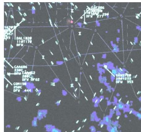
Figure 3 Air Traffic Controllers Display with NEXRAD Radar
