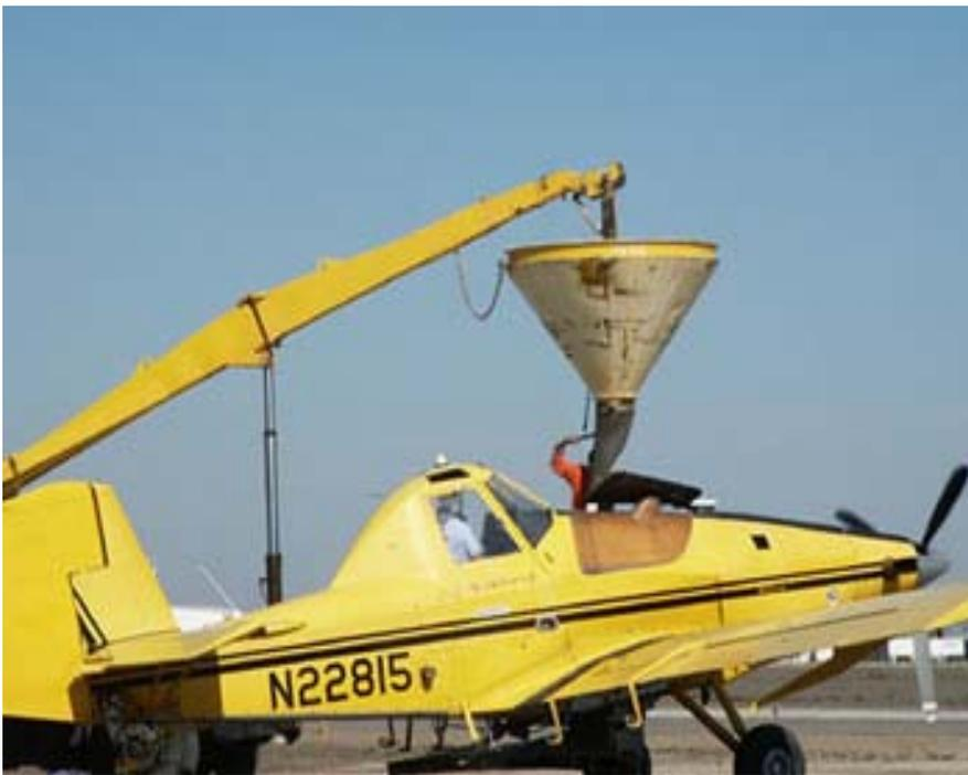
Figure 1: Turbine Thrush Commander being loaded with fertilizer at Corcoran, CA
