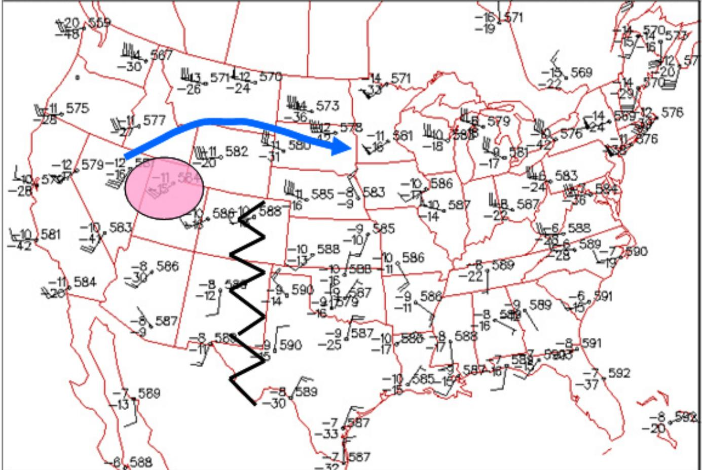
**Figure 2.** 500 mb chart valid 12 UTC 09 July 2004. Station plots contain the following data: temperature (°C) top left, dewpoint (°C) bottom left, geopotential height (decameters) and winds (pennant, full barb, and half barb denote 10, and 5 kts, respectively). Blue arrow (500 mb jet axis), pink oval (right rear quadrant of jet) and black zig-zag is the 500 mb ridge axis.
