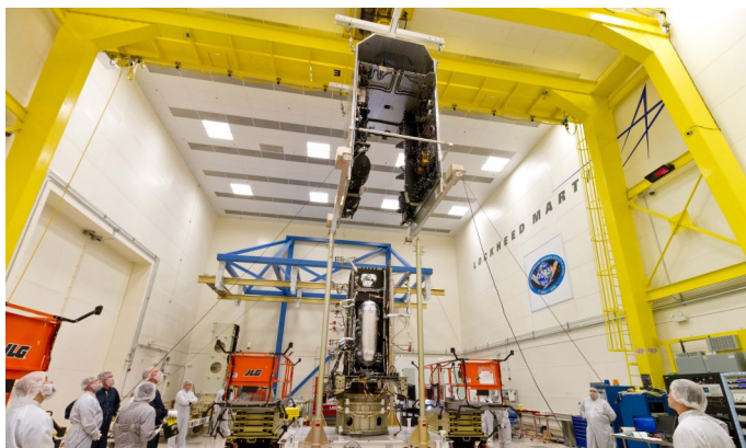
The GOES-R spacecraft "body" (lower portion) is mated with the "brain" of the satellite in the clean room of Lockheed Martin near Denver, Colorado, on Sept. 6. Photo Credit: Lockheed Martin
