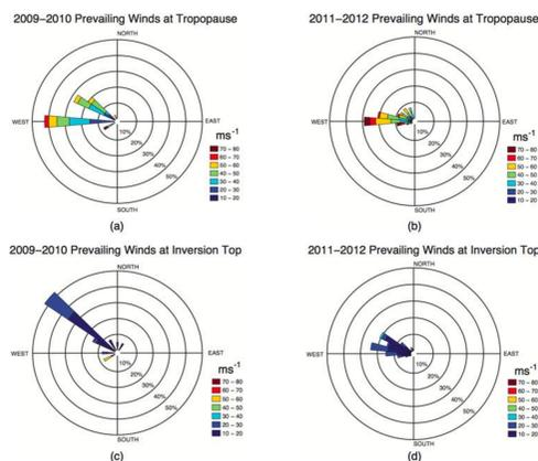
Figure 2: Wind roses for 2009-2010 (left) and 2011-2012 (right). Frequency and strength of wind speed and direction at the tropopause (top) and at the inversion top (bottom).
