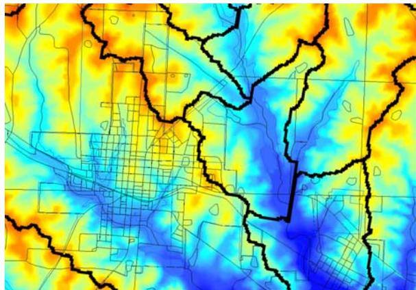
Figure 7. Digital Elevation Map of Sylvester, Georgia with KTLH FFMP basin vectors in black.
