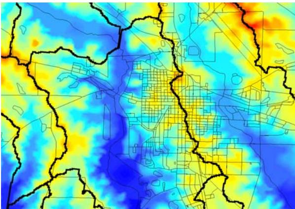
Figure 6. Digital Elevation Map of Moultrie Georgia with KTLH FFMP basin vectors in black.
