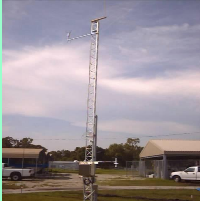
Radiosonde Surface Observing Instrumentation System mast and attached sensors, at NWS Tampa Bay Area in Ruskin.
