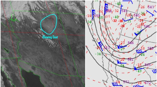
Figure 2- 1715 UTC visible satellite imagery (left), and 00Z April 4<sup>th</sup> 500 mb analysis (right) depicting strong southwest flow ahead of approaching shortwave trough.
