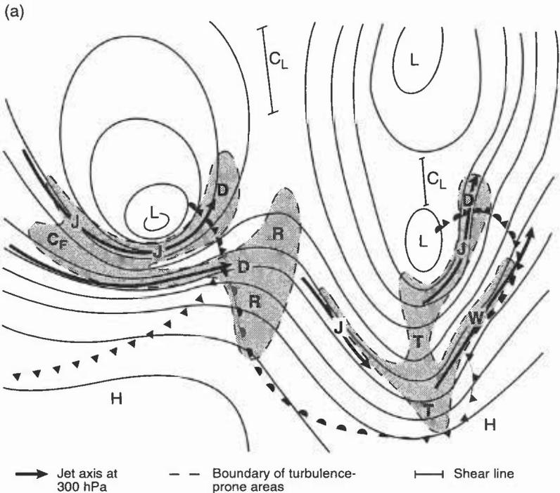
**Figure 6.2(a).** Main turbulence-prone areas between 500 and 200 hPa as related to features of the 300 hPa chart.
