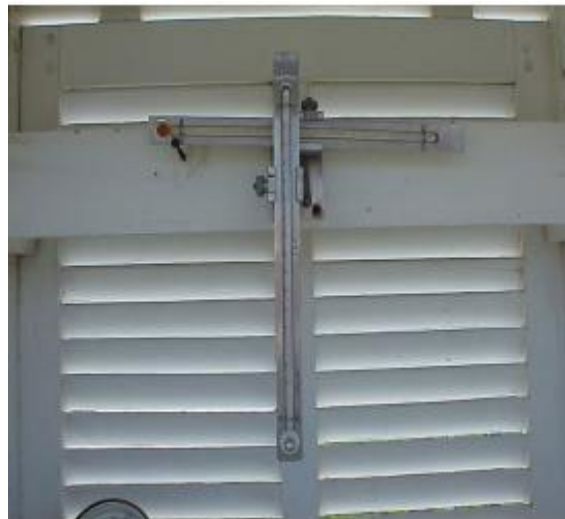
Figure B-30. Maximum Thermometer in Reading Position
