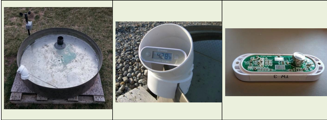
Figure A-30. Position the Tip of Probe into Shaded Side of Pan
