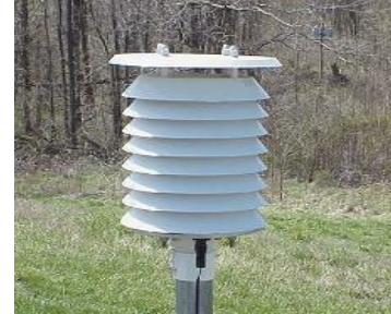
Figure A-13. MMTS Shelter
