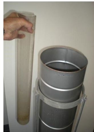
Figure B-10. Removing the Measuring Tube
