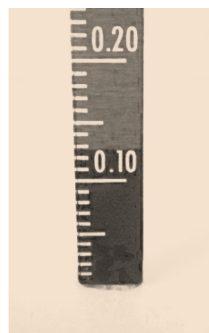
Figure B-13. Reading the Precipitation Amount (0.13)
