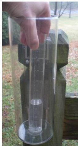
Figure B-6. Removing the Measuring Tube
