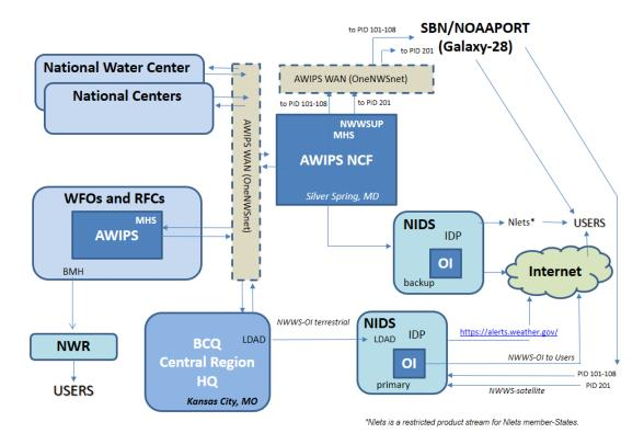
Figure 3.1 NWWS Enterprise Architecture Diagram; product flow
