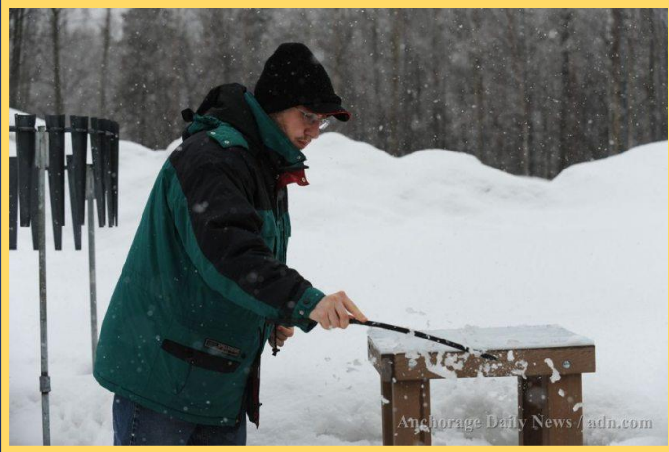
NWS meteorologist clearing snow table after a measurement
