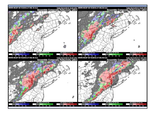
1700 UTC 2018-05-15 run of the HRRR. Ensemble composite reflectivity forecasts show that the 1500 UTC and 1600 UTC runs of the HRRR develop convection too far North with the 1700 UTC run developing the convection slightly further south. The 1700 UTC run 1-hour forecast valid at 1800 UTC is underdone with respect to the initial supercell convection.
