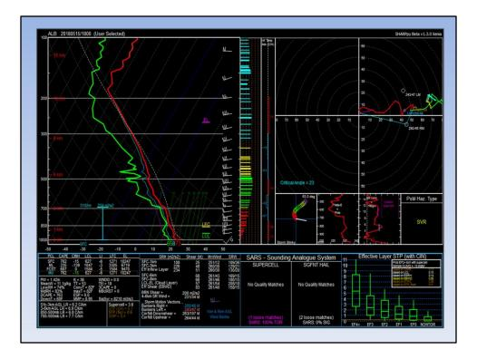
18Z sounding at Albany, NY displays CAPE < 1000 J/kg, effective shear > 80 kts, effective SRH > 200 m^2/s^2 and mid-level lapse rates > 7.5 C/km.
