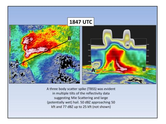
KENX reflectivity cross section of the Saugerties supercell at 1847Z reveals a bounded weak echo region (BWER) suggesting a very strong and persistent updraft. A three body scatter spike (TBSS) was evident in multiple tilts of the reflectivity data suggesting Mie Scattering and large (potentially wet) hail. 50 dbz approaching 50 kft and 77 dbz up to 25 kft (not shown).
