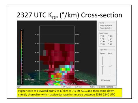
2327 UTC KENX KDP cross-section shows a higher core of elevated KDP aloft of 5 to  $6^{\circ}$ /km to 7.5 kft AGL, and with values of 4-5 $^{\circ}$ /km to close to 12 kft AGL.
