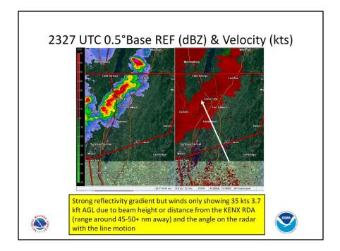
At 2327 UTC, the KENX radar imagery zoomed in, shows a strong reflectivity gradient, but the 0.5° velocity data only shows 35 knots 3.7 kft AGL due to the beam height/distance from the RDA (range of 45-50+ nm), and the angle on the radar with the line motion. This area was near the macroburst.
