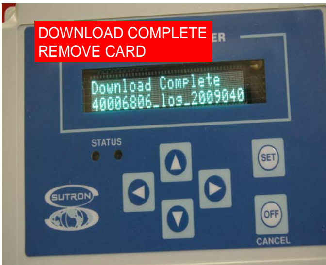
Figure 2. The message Observers will see when data transfers between the computer and the SD Card. ■
