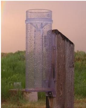
*Left: A 4-inch diameter rain gauge that CoCoRaHS observers use to collect rainfall. The large diameter allows a representative amount of precipitation to filter into the gauge so observers can record an accurate total for each event.*
