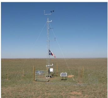
The stations stand at over 30 feet tall and are located away from the city, trees, hills, and other features that could interfere with the meteorological instruments. More information and weather data from these site and others can be found at the West Texas Mesonet website at <a href="https://www.mesonet.ttu.edu">www.mesonet.ttu.edu</a>. Below is a map of most of the mesonet stations that the West Texas Mesonet is currently operating and maintaining.
