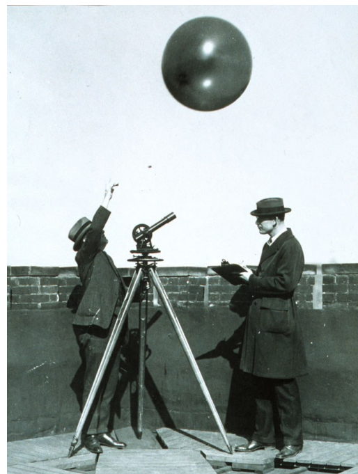
This image shows early testing of hydrogen-filled balloons for radiosonde measurements. The theodolite in the image was used to track the balloon to the limit of visibility.
