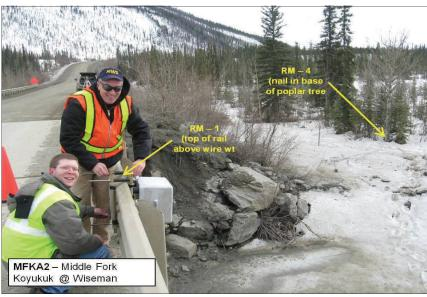
Forecaster Ray Little (left) and Observation Program Leader Brad Sipperly perform routine maintenance on a wire weight gage located on the Middle Fork of the Koyukuk River. Both Ray and Brad work in the Fairbanks WFO.
