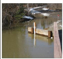
changes in water levels from specific points within the community, which was extremely important for emergency response and evacuations. The addition of these gages will help to forecast and prepare for future floods in the Salcha area.
