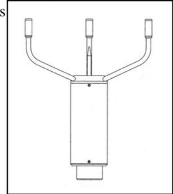
The Vaisala 425NWS Ice Free ultrasonic wind sensor is an array of three equally spaced transducers which radiate and receive ultrasonic pulses in a horizontal plane. The sensor measures transit times in both directions for each of the three transducer pairs. The wind speed and direction are then derived from these six transit time measurements.
