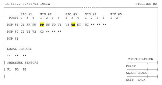
Figure 3: SENSOR CONFIGURATION Page (REVUE-SITE-CONFG-SENSR).
