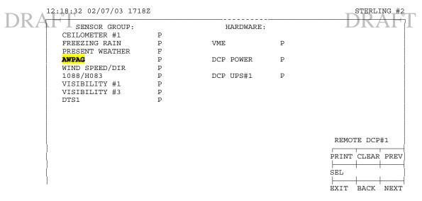
Figure 10: ACU / Remote DCP STATUS Page (MAINT-DCP#1)1
