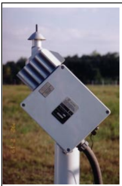
Figure 17. Freezing Rain Sensor
