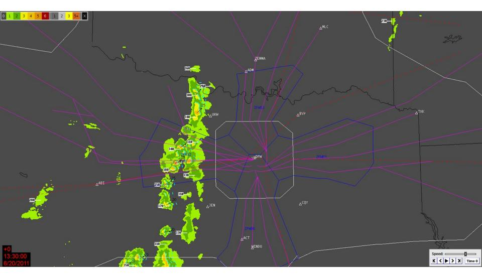
NEXRAD GR Analyst imagery at 12:52z 6/20/11 indicated narrow broken line of mainly elevated SHRA/TS West of D10. Virga bases were around 090-150 as noted in circled area of 3D rendering with most convective elements at or below 40 dBZ.
