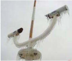
Ice accumulation on the Lexington ASOS visibility sensor during the historic ice storm of February 2003.
