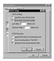
Select Echo typed characters and click the OK button to close the windows. The program is now set up to communicate with the Nimbus PL Thermometer. The command set may be retrieved using command at?
