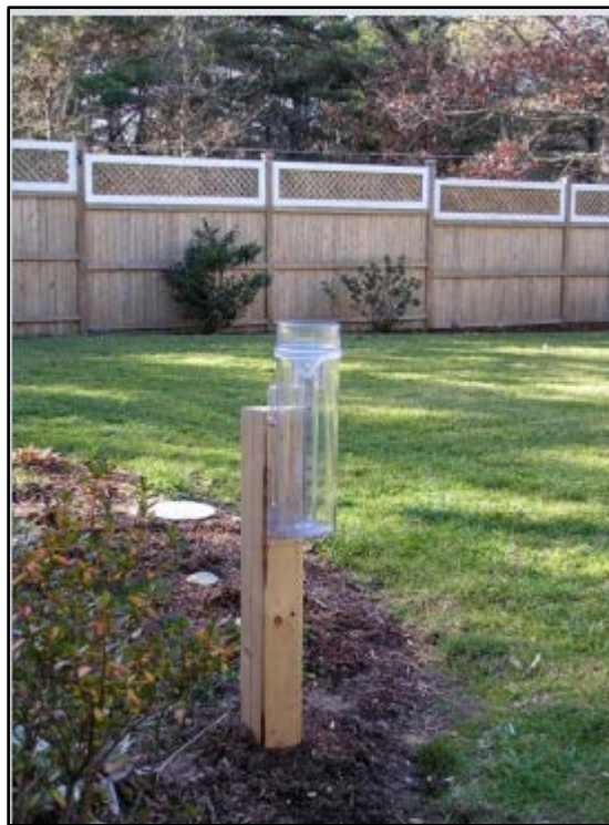
Photo of a CoCoRaHS rain gauge.
