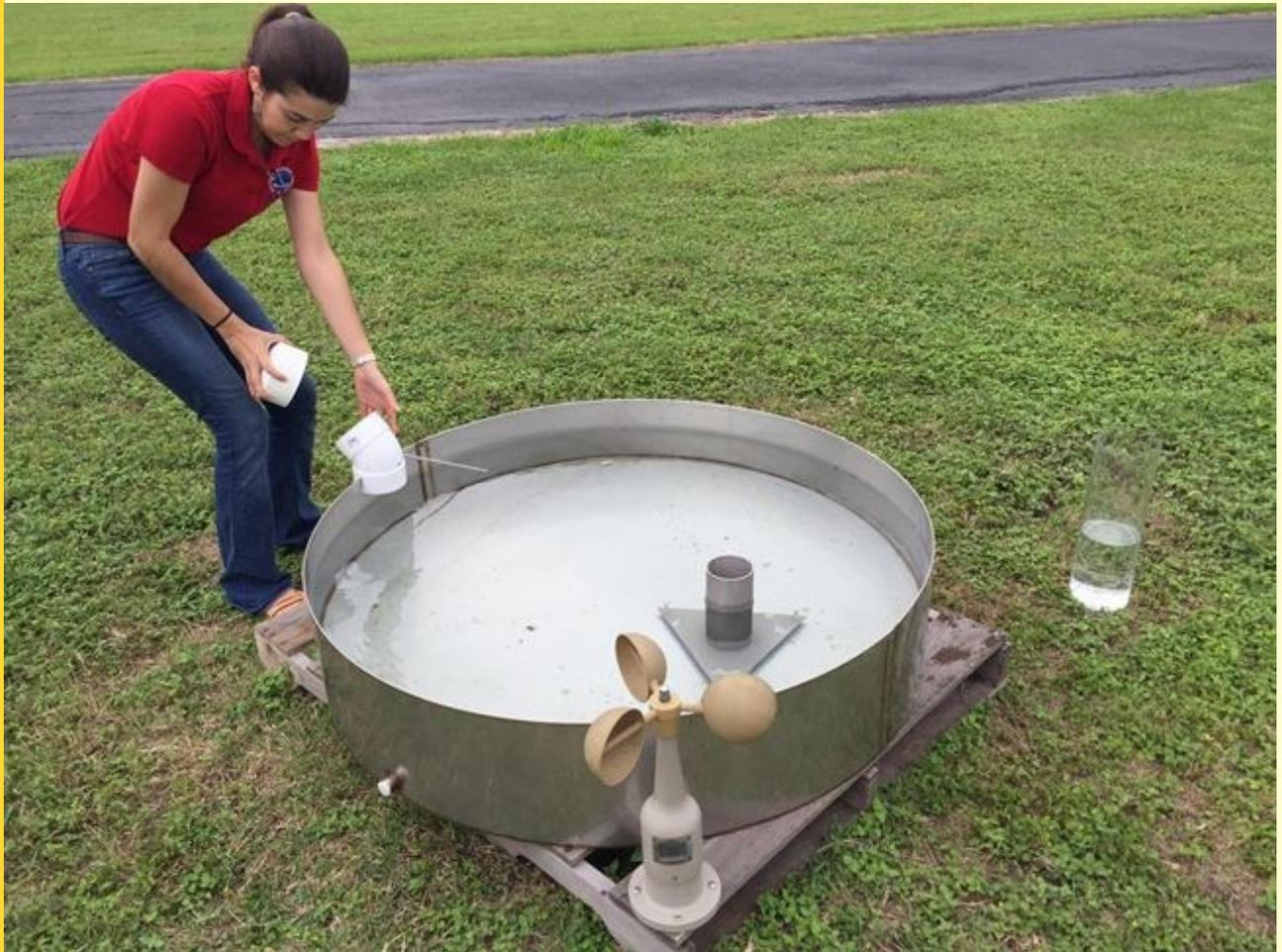
**Above:** The giant pan, seen in the picture with Forecaster Maria Torres, is full of water that we use to measure the displacement of water each 24-hour period. We also measure the amount of wind that flows over the pan each day, which can have a substantial factor on evaporation rates of soil.
