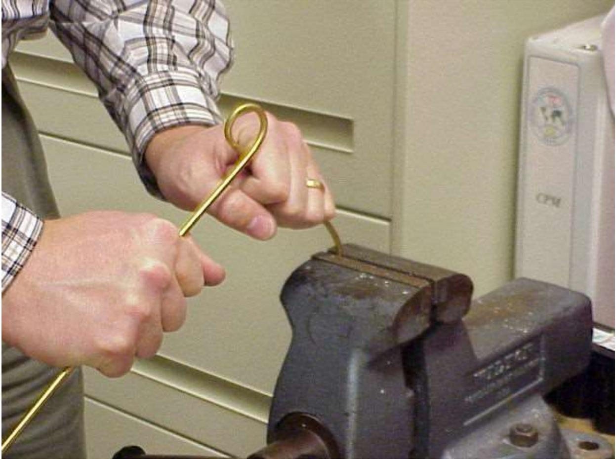
Measure 10" in from each end, and bend the rods so that when you hold the rod by the loop in the middle, the bent rod ends point straight down.
