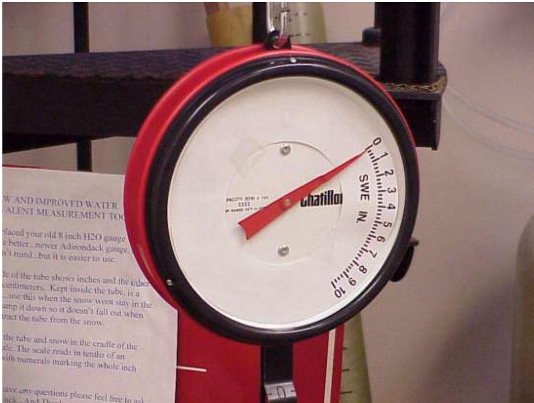
Most scales have an adjustment screw on the hanger to fine tune the zero reading. Read the instructions with your unit.
