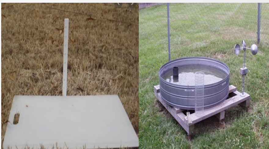
Snow board, snow stick, and evaporation pan
